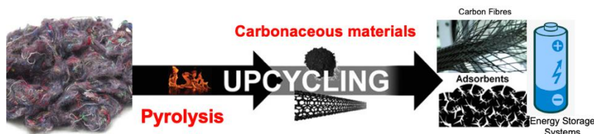
Fig. 1. Upcycling of Fibrous wastes to Carbon-based functional materials.
